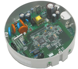
Meter Interior showing muNet IP Interface Communication Board
